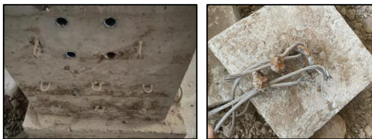
(a) 桥台试验后状态
