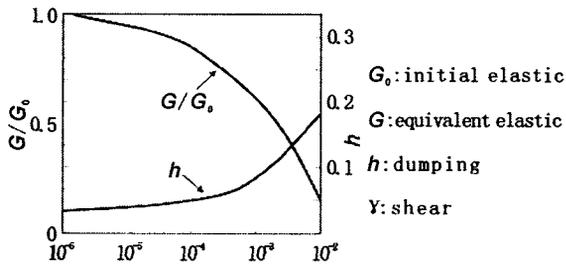
Fig. 5 Equivalent linearization of elastic shear coefficient  $G$  and damping constant  $h$ .
