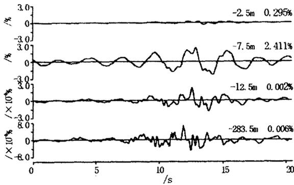
Fig. 9 Shear strains in depth at the 2<sup>nd</sup> port.
