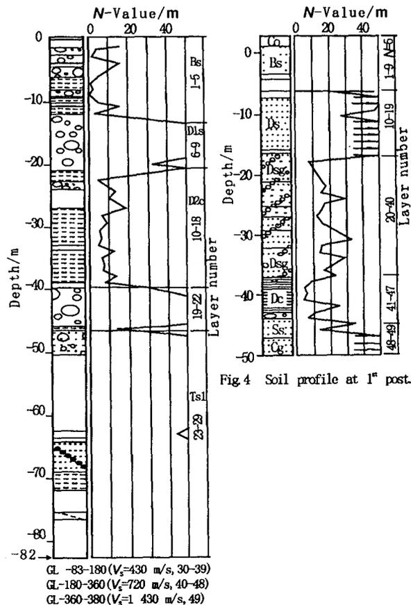
Fig. 4 Soil profile at 1<sup>st</sup> post.
