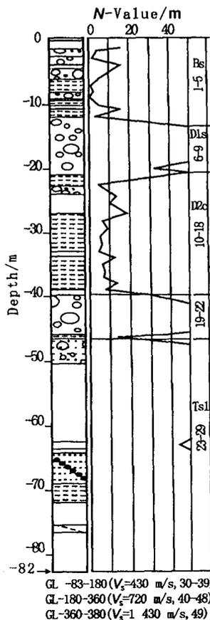
Fig. 3 Soil profile at 2<sup>nd</sup> post.
