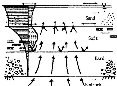
Fig. 1 Concept of mechanism of liquefaction.
