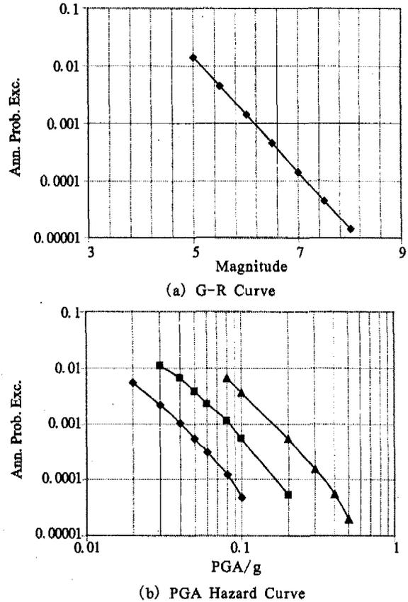
Fig. 4 Gutenberg-Richter (a) and PGA (b) hazard curves for a site 40 km from a line source (Square; median; diamond; median  $- \sigma_{ln,y}$ ; triangle; median  $+ \sigma_{ln,y}$ ).
