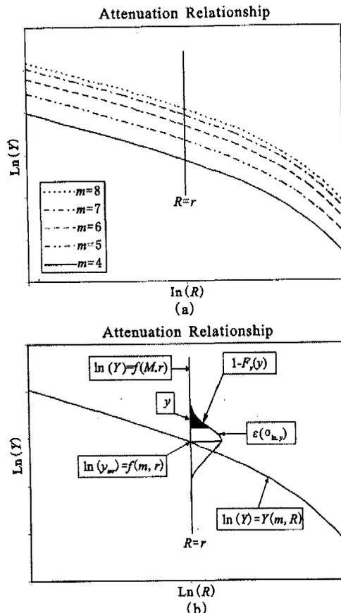
Fig. 2 Ground-motion attenuation relationship (a) and ground-motion uncertainty at a given  $m$  and  $r$  (b).
